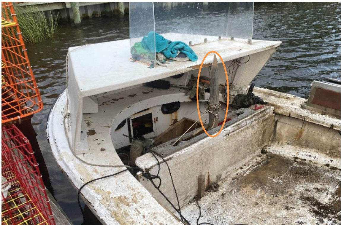
Figure 5: Photograph of the operating area in the bow of NC3250BW. The oval highlights the tiller handle used for steering from the forward position of vessel. Photo sourced from the USCG Investigating Officer.
