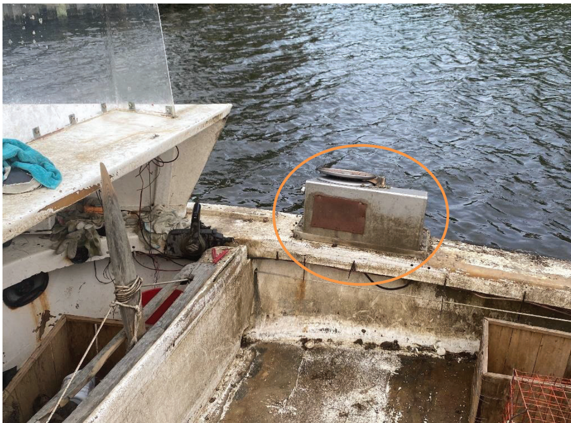
Figure 6: Photograph of operating area of NC3250BW. The circle highlights the “pot puller” mounted on the starboard gunwale. Photo sourced from the USCG Investigating Officer.
